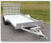
DOT Approved, LED Lighting System, Tires: ST205/75D14, White Powder Coated Rims, Torsion Axle, Coupler: 2"x3", 3500lbs Coupler, 750lbs Jockey Wheel
